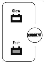
STEP 3: Press "CURRENT" button to select "Slow" or "Fast" charging current ("Slow"-green light, "Fast"red light) (6V/2A,12V 2A/15A). If you choose 12V LiFePO4 in STEP 2, the default current will be "Fast". You don't need to select charging current and battery type.
