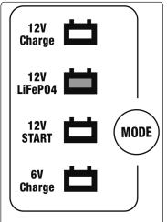
STEP 2: Press "MODE" button To select charging voltage (6V/12V) (orange light, except 12V START).
