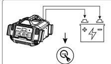
**STEP 3:** The charger starts to charge the battery automatically.
